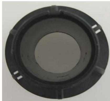
NOTE: The P17, B17, and SS577 (2" diameter) housings do not have a built-in valve. The valve sleeve (shown above) is separate from the housing. The installer slides the valve sleeve into the housing during installation.
